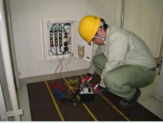
measured by voltage drop method with 500Hz constant current
