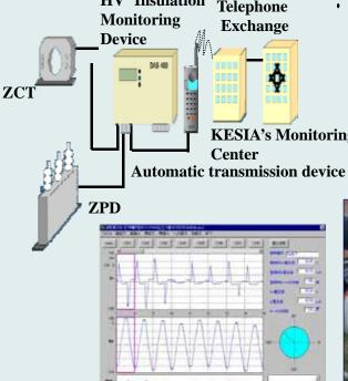
Telephone<br/>ExchangeRegular monitoring of zero-phase<br/>voltage, zero-phase current, lo<br/>pulse, wave profile, and<br/>grounding resistance enables<br/>early detection of precursory<br/>effect of slight ground faultKESIA's Monitoring<br/>Centerbefore the real earth fault occurs,<br/>to prevent a HV grounding fault
